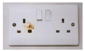
Sockets can be damaged by faulty appliances or plugs overheating. The socket outlet will need to be replaced and the electrics checked if there are any sign of overheating (example left).
