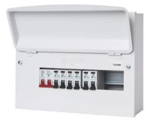
This is a typical domestic Consumer Unit (CU) also known as a Distribution Board. It connects and distributes to the incoming electrical supply to the various circuits in the property. You will find a number of the outer cabinets are made out of plastic but the 18<sup>th</sup> edition of the IEE Regulations now require the cabinets are made from a noncombustible material and so newer cabinets are commonly made from steel.
